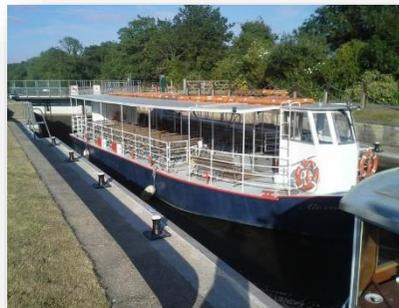
This vessel is 62 ft in length and has a beam of 17'6. with a total square footage of 864 sq.ft. The hull is constructed from steel and completed 1979. Presently there is a Ford diesel 108 6 cylinder engine in place, there are 2 toilet compartments. Below decks there is a soil tank, water tank and fuel tank and ample additional dry storage.
